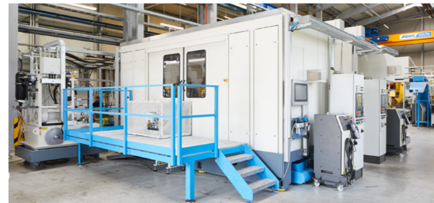
At right: an HSTA 550-4 for flow forming of the rim rings. A central robot relays the workpieces from one machine to the next.
