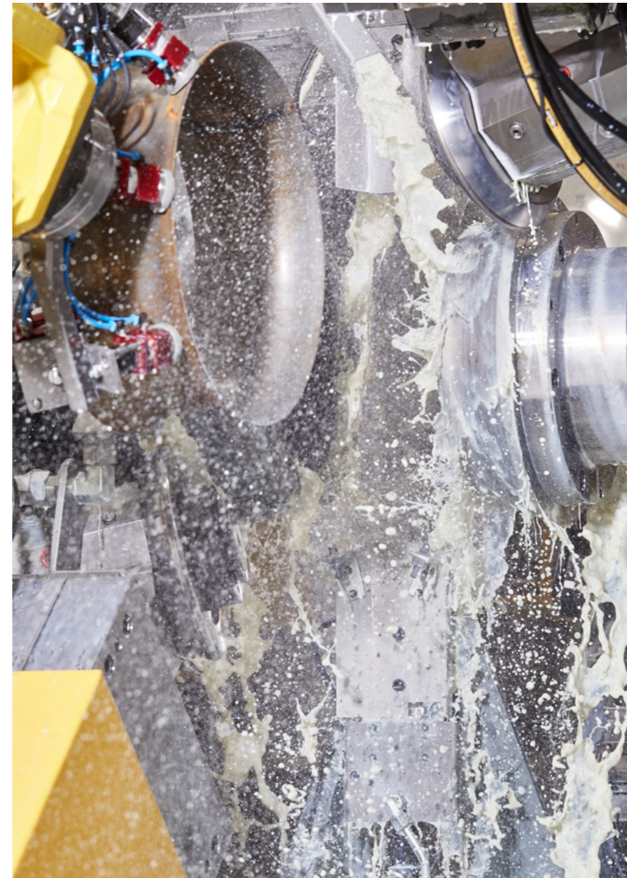
The discs are trimmed and deburred on an HABS during a second operation.
