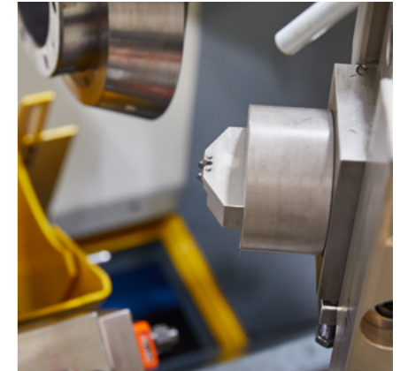
The discs are trimmed and deburred on an HABS during a second operation.
