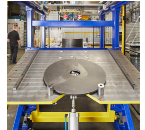
The blank de-stacking unit singles staples of up to 3x40 blanks and feeds them to the robot.
