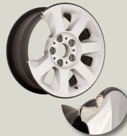
The hybrid wheel – a combination of aluminium front face and a steel rim
