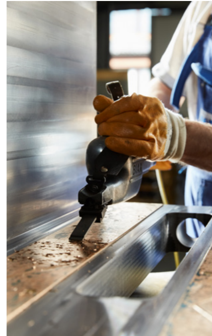
Hand-made bronze guideways – a WF quality feature
