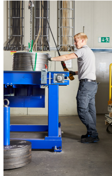
Simple positioning of stapled blanks
